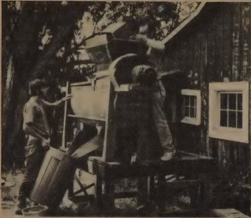
Those who make large quantities of wine may want to employ some sort of a mechanical stemmer-crusher. This is an ancient model at Phil Palmer's home. Mike Palmer is emptying a lug of grapes. Stems shoot out the far end. The pulp and juice come out the spout into the plastic garbage container in which fermenting will take place.
